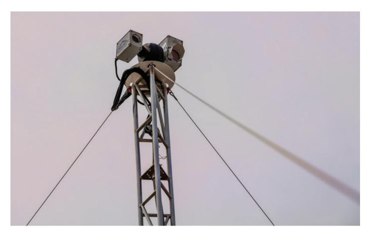
Figure 7: A close-up shot of LongPath's Continuous Open-Path Sensor, which utilizes invisible, eye-safe long-range lasers to detect methane-specific greenhouse gas molecules up to a 2.5-mile radius from installation.
