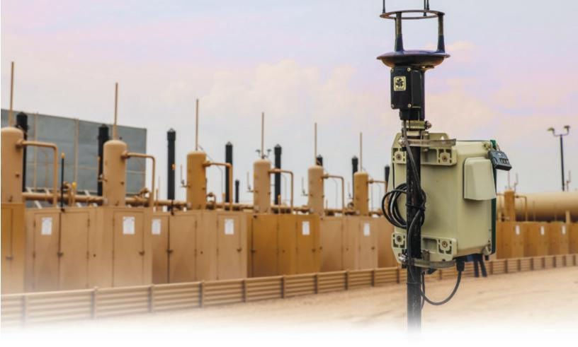
Figure 5: A Project Canary monitoring device located on one of Bayswater's Colorado production sites.
