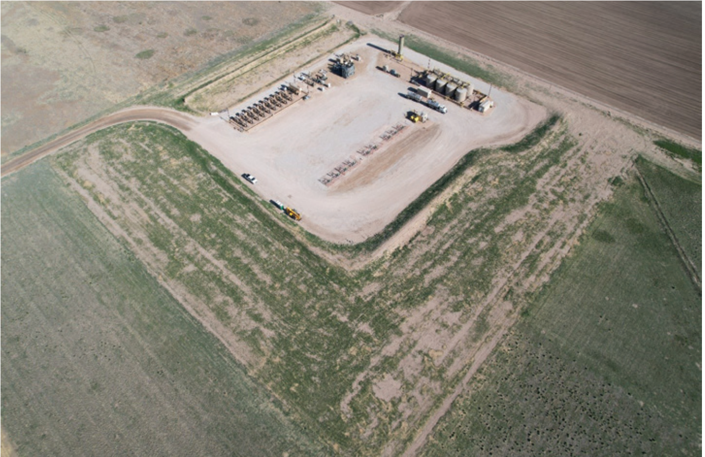
Figure 20: An example of interim reclamation conducted on Bayswater's Groves pad in the DJ Basin. Native vegetation has significantly regrown in the interim reclaimed acreage, but the original footprint of the pad during drilling and completions is still just visible.
